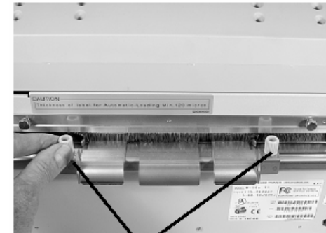
Label Width Adjustment Thumbscrews
